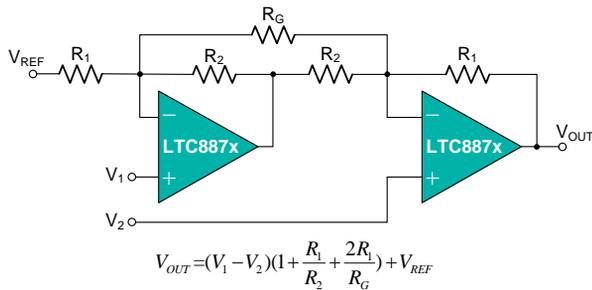
Figure 9. Instrumentation Amplifier
