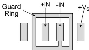
Figure 4. Use a guard ring around sensitive pins
